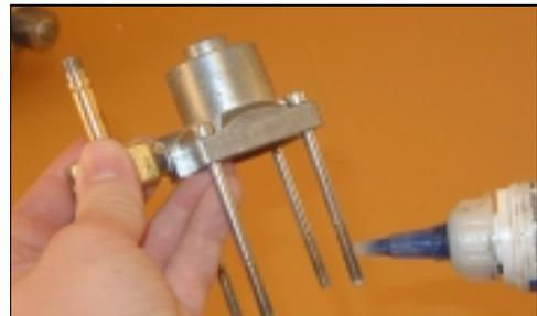
18. Place the valve actuator housing with the new O-ring on the valve plate, using your hand to guide it into the correct position.
