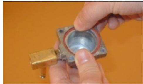
17. The new valve actuator housing is now ready to be attached to the valve plate, but first of all place a little Loctite # 243 on the four screws.
