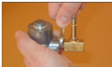
15. Turn the solenoid valve housing until the distance between the solenoid valve and the valve actuator housing is approximately 13/64 inch (5 mm) and the spool points directly upwards in relation to the valve actuator housing.
