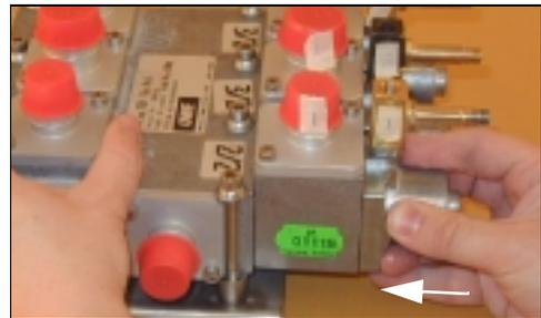
19. Screw the Allen screws loosely to make it easier to fit the Banjo couplings. These screws must be torqued in step 25.
