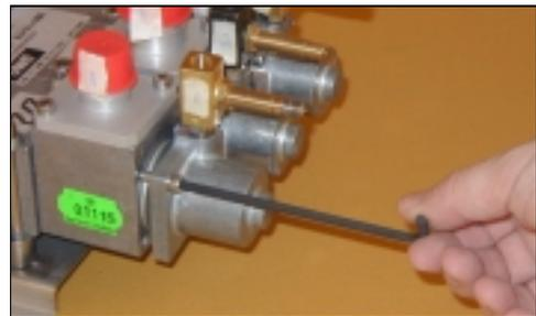
8. Lift off the valve actuator housing.
