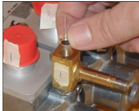
22. Place the Banjo bolt in the Banjo housing with the two bonded seals as shown in figure right.
