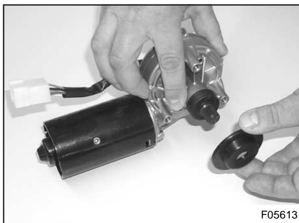
Figure 11 : Wiper motor dust cap installation (for the sake of clarity shown with the motor out of the coach)
