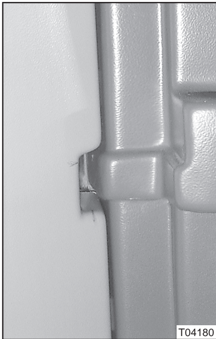
Figures 1,2 and 3: Glare shield fitted to upper front inside corner of driver's window frame (T2100 Series-Overall view and detail)
