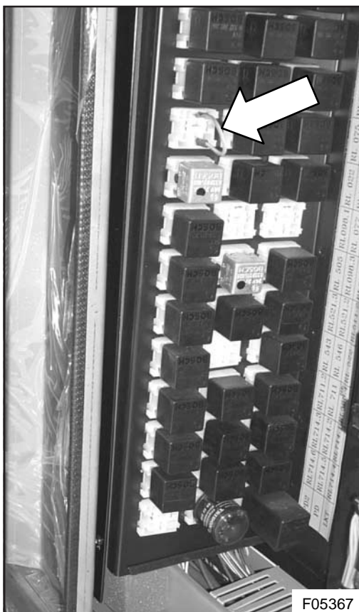
Figure 1 : Location of RL75 relay holder with jumper wire
