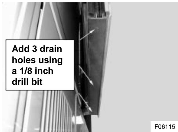
**Figure 27: Sliding lift door drain holes**
