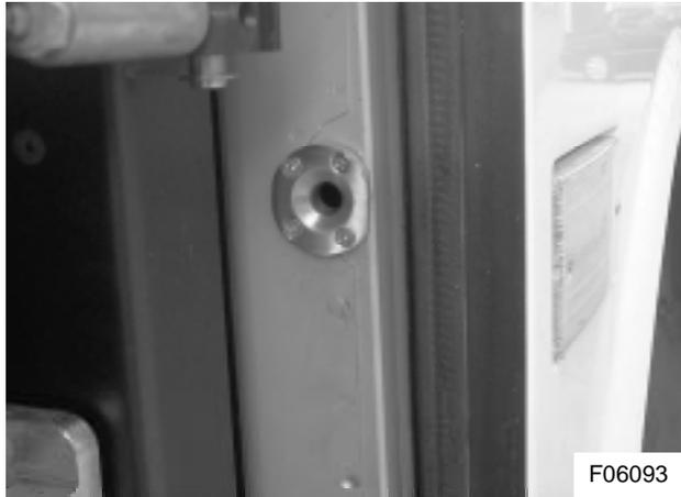
**Figure 39: New guide pin catch installation**
