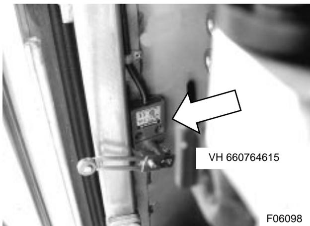
**Figure 45: Old location of proximity switch VH 660764615 next to lift compartment side post**
