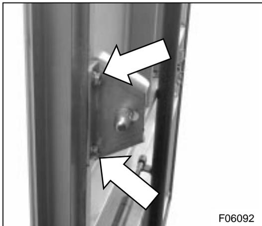
**Figure 37: Guide pin brackets and mounting bolts**
