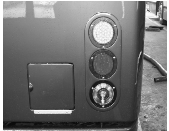
Figure 4: Right hand rear light cluster installation completed
