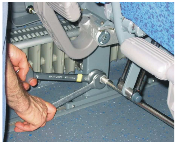
Figure 13: Adjusting the push/pull rod throw
