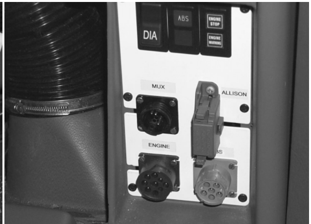
Figure 8: Diagnostic plug (located below right hand dash panel)
