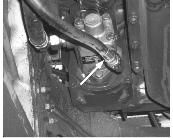
Figure 6: Beneath the coach at the rear - C2045 and T2145 w/ Cummins engine - pressure feed line at hydraulic pump. Check one crimp fitting.
