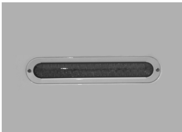
Figure 1: High mount stop lamp on US coach (typical installation)
