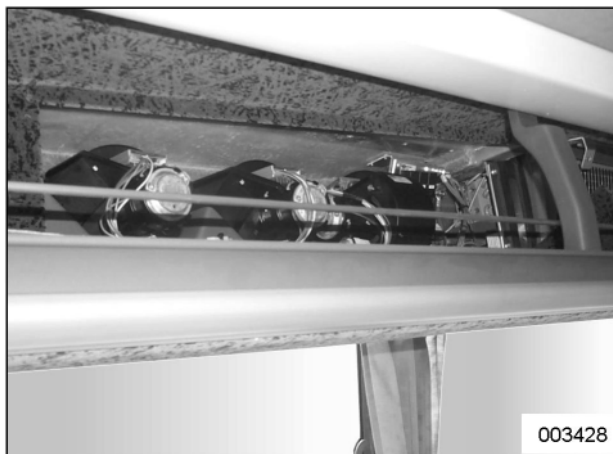
Figure 4: T2100 evaporator blower bank (left-hand)
