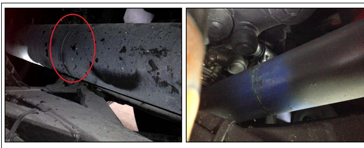
Figure 1: Location of interference damage
