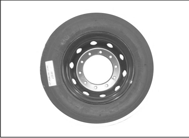
Figure 1.1: In production the wheel to hub mounting surface are masked off before painting
