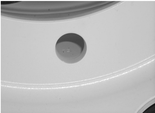
Figure 1.3: OE supplied wheels come in two colors - white and silver. Paint thickness has been established at a total of 2.36 mils
