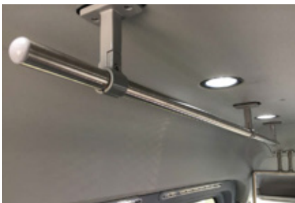
Ceiling mounted grab bar and overhead lighting.
