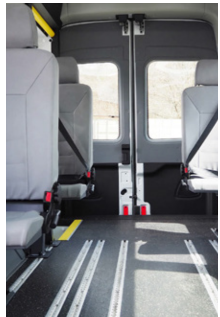
Wide aisle room for ambulatory riders and wheelchairs with easy access to rear walk-in door.
